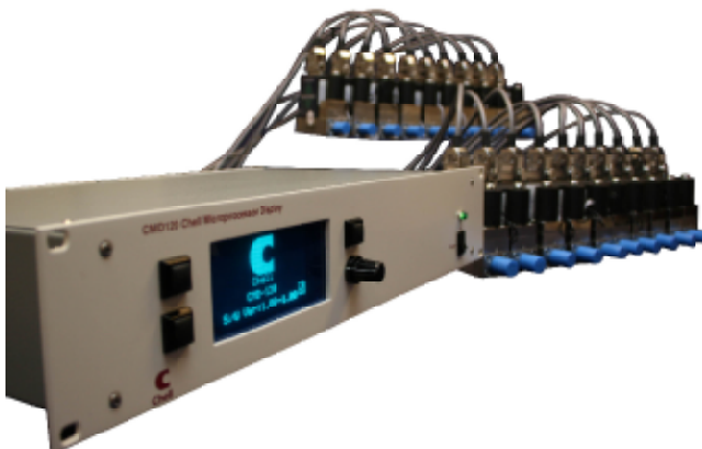
Chell CMD120 supplied with 20 Hastings MFC's
