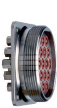
SQDC-S-19-20-S 19 way bulkhead half, Standard seal configuration, compression fittings and ferrules for 1/16 inch tubing. Silicon seals
