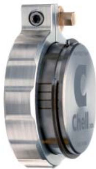
SQDC-S-19-05 19 way removable half blank, Standard seal configuration. All ports sealed.
